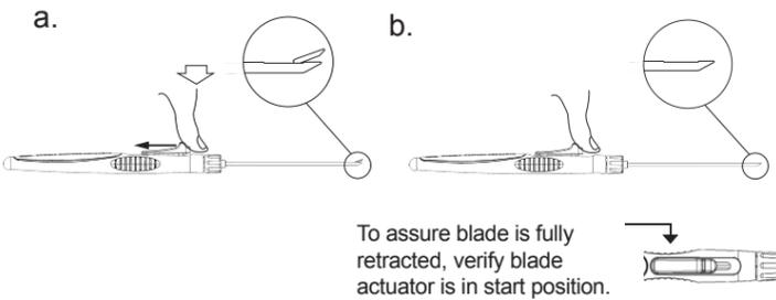
3. To insert or remove device, ensure blade is completely retracted:
