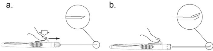
2. To retract blade, depress blade actuator and push away from tip of device.
